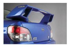
Cosmetic body modifications such as side skirts and front/rear spoilers are permitted without DPTI approval provided that they are fitted with regard to the safety of other road users. They must meet ground clearance requirements of 100mm. It is recommended that air flow for brake cooling is not adversely affected.
