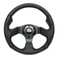
Passenger vehicles built after 1970 are required to comply with ADR 10. The replacement steering wheel must have the appropriate markings indicating that it complies with ADR 10. There are a number of steering wheels certified to ADR 10, so prior to purchasing an aftermarket steering wheel contact Vehicle Standards to ensure that it is acceptable.
